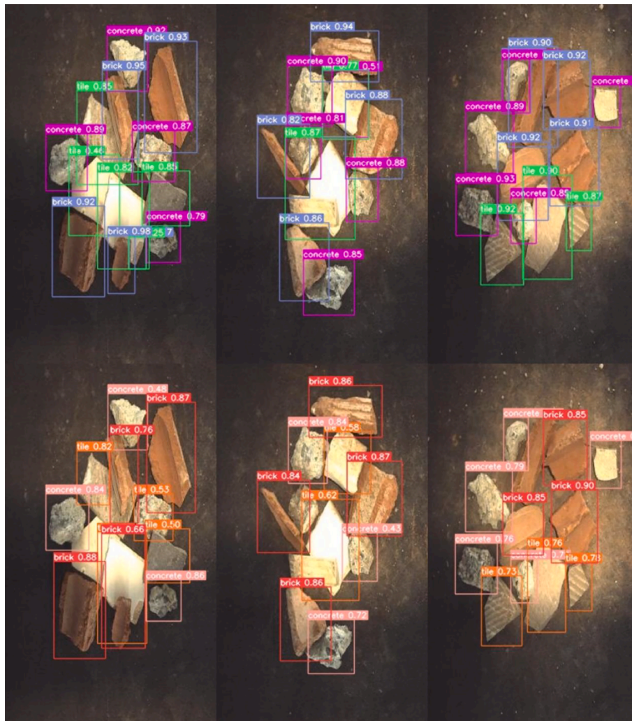
Fig. 7. Inference results on testing set_2 from YoloV7x model (top), YoloV5l model (bottom).
