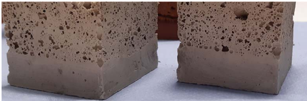
Figure 2. Small-scale DEF-EAT-CM prototypes based entirely on waste ceramic tiles (CTFR-CTTI).
