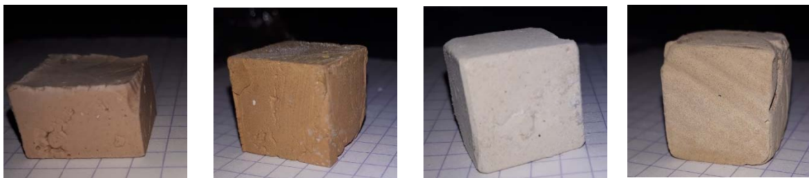
Figure 9: Binder samples after 2 h exposure to 1100 °C. From left: IP tiles, IP bricks, blended cements tiles, blended cement bricks.
