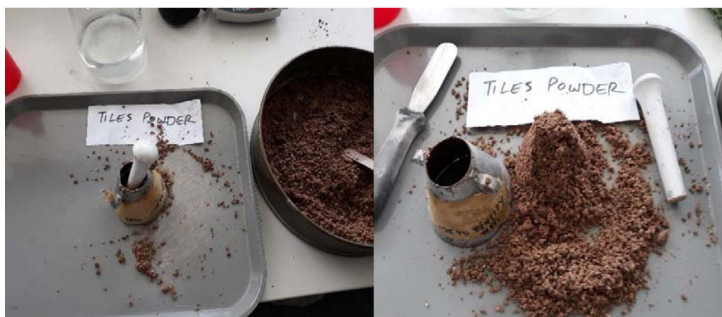
Figure 21. The sample tested in a saturated surface dry condition (right picture).
