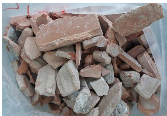
Figure 12. The raw materials as received from CDW (waste brick).
