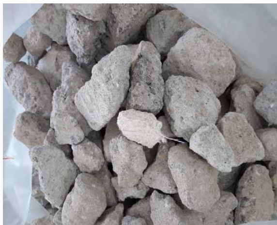
Figure 14. The raw materials as received from CDW (waste concrete).
