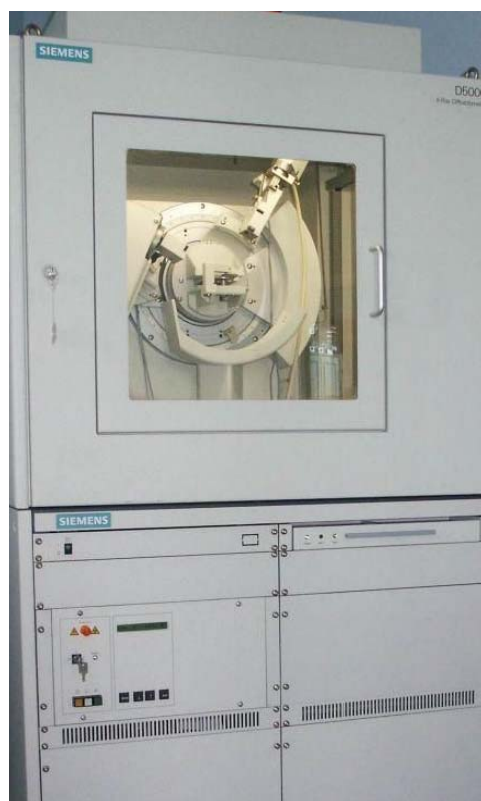
Figure 8. The SIEMENS D5000 X-ray diffractometer used in the experiment.
