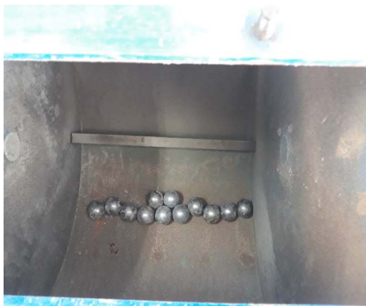
Figure 16. The stainless balls inside the Los Angeles abrasion machine.
