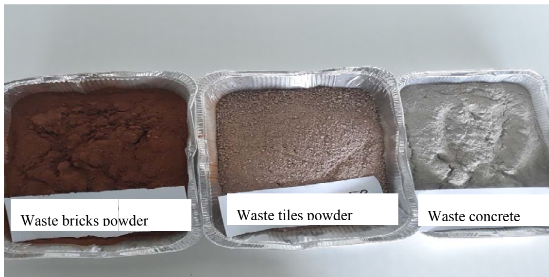
Figure 18. The ground raw materials from CDW.
