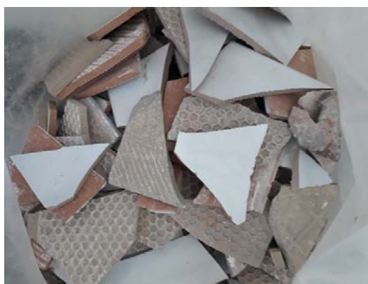
Figure 13. The raw materials as received from CDW (waste tiles).
