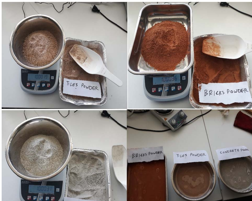
Figure 19. Weighing and immersion of samples.
