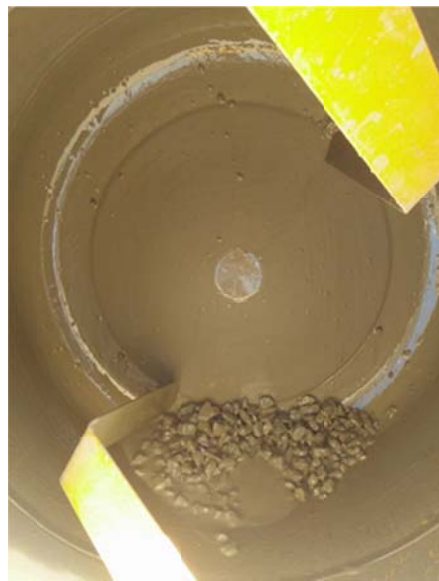
Figure 2. Treatment of Recycled Concrete Aggregates (RCA) in 100L concrete mixer for treatment.
