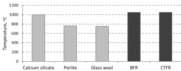
Fig. 2. Maximum temperature of application for typical insulating materials used also as fire resistant [24] (BFR and CTFR are the geopolymers developed in this study).
